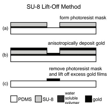
**Figure 1.** Lift-off method using SU-8 as the photoresist, water-soluble polymer (PAA) as an intermediate sacrificial layer, and DI water as the terminal stripper. Thin-film gold is anisotropically deposited using an electron beam evaporator.
