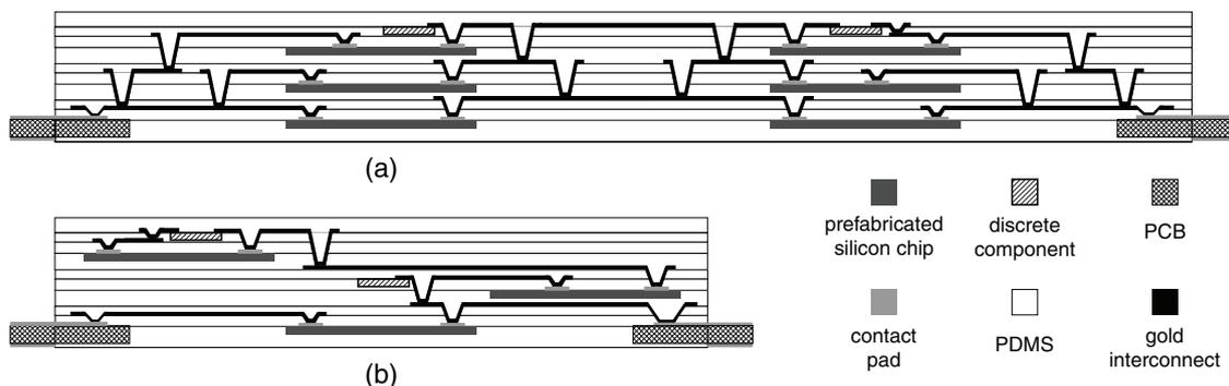
**Figure 4.** Architecture for an elastic, multichip module (not to scale). PCBs, prefabricated silicon ICs, and thin-film discrete components of various types can all be integrated into such a composite and interconnected using multilayer via-bonding technology to form a module-level circuit. (a) Components aggregate in stacked 3D islands. This architecture can maximize the system-level stretchability. (b) Components are not stacked. This architecture gives more design flexibility.
